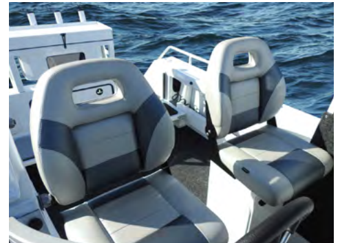
Two folding seats with a marine grade alloy hinging. PRO DECK™ has aluminium seat boxes w/ hatches.
