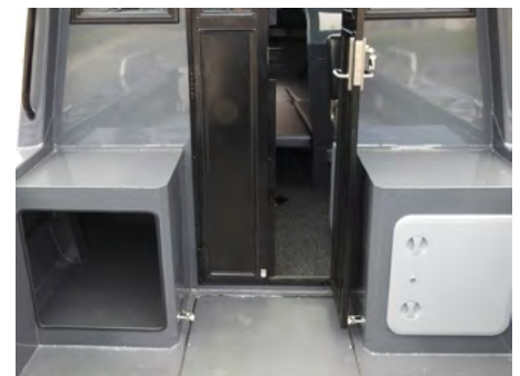
Large seat boxes with storage that extends out to the rear deck.
