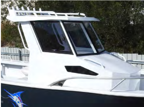
Fixed Glass Windscreen, sliding side windows. Fixed Hardtop, handrails and rocket launcher.
