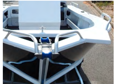
Standard: Electric Motor Mount, Bollard, Heavy-duty Bowroller, Aluminium Anchor Well, 32mm Handrails.
