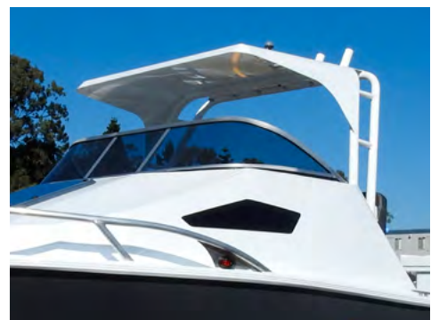
OPTION: Folding Rocket Launcher with heavy-duty extrusions and aluminium visor.
