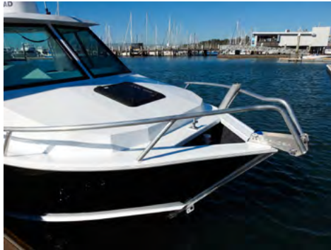
Large cabin hatch for access to aluminium anchor well and bowroller. Tube is an option.
