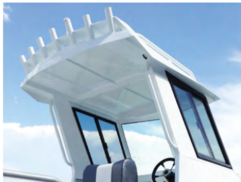
Enclosed Centre Cabin Hardtop with Radio Box, Rod Holders and handrails.
