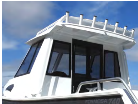
Fixed windscreen, sliding windows, lockable doors with Rocket Launcher and grab rails.
