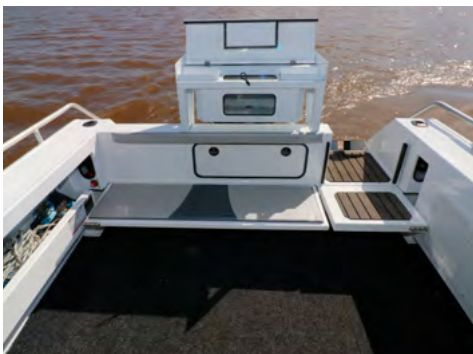
Rear 3/4 flush folding rear lounge w/ backrest, transom hatches, battery access are standard.
