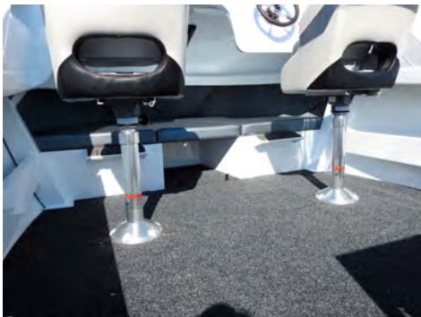
Air Ride Pedestals with adjusting gas lever. Powder coated aluminium swivel.
