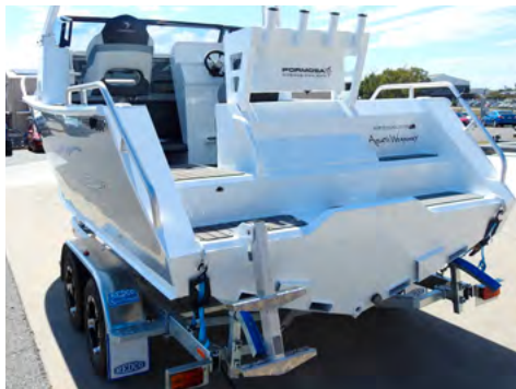
Single Access Active Transom w/ 2-step heavy-duty ladder and right grab handle are standard.
