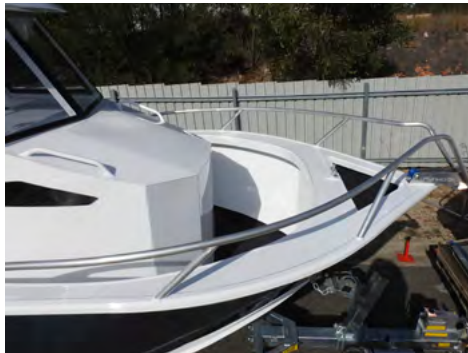
Walk around Cabin with raised casting deck, aluminium anchor well, handrails and bowroller.
