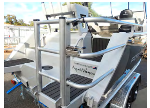
OPTION: Transom Casting Cage with extended casting platform, dual or single available.
