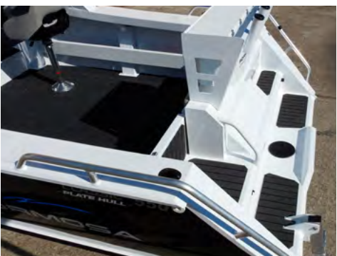
Single Access 'Active Transom' is standard with flush folding transom door. Step down transom, internal grab rail, heavy-duty dive ladder.
